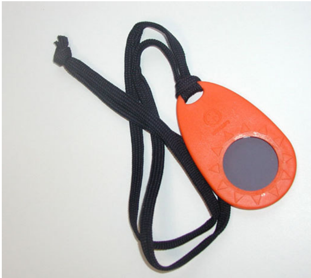
Sunsure: this simple filter 'tells' sunbathers when it is time to get out of the sun.
