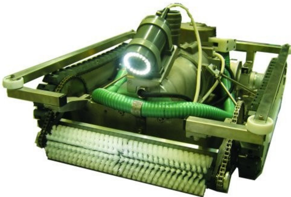
The underwater cleaning robot, with camera attached
